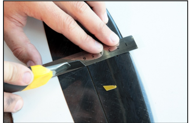
Figure 2.1 - Bonding elevator horn
